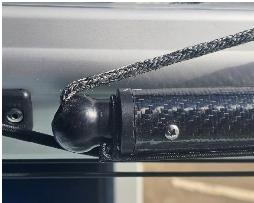
Elastic tied to inner end of pole
