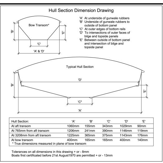
When a straight edge is placed upon either topsides, side decks, bilge panels or centre bottom panel in the same plane as the sections, no part of the surface shall be further away from the straight edge than 3mm.
